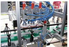
• Multi-head 4L round head tester with offset neck orientation. This was for a steel container.
